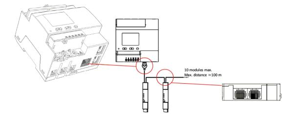
Important note: Each EMS module is supplied with an ESY bus termination (see the picture below).
